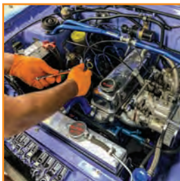
Crow foot sockets for hard-to-reach nuts and bolts
